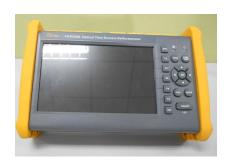
Name: optical time domain reflectometer(OTDR)
