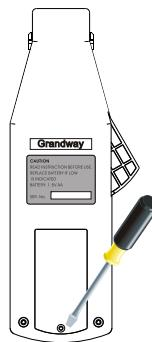
**Note:** 1 It is advisable to use 1.5V alkaline batteries. The Low Battery Indicator may light up if you use rechargeable batteries.
