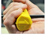
Close the tool onto the cable and pull in the direction of the arrow; clamps tightly — no latch required.
