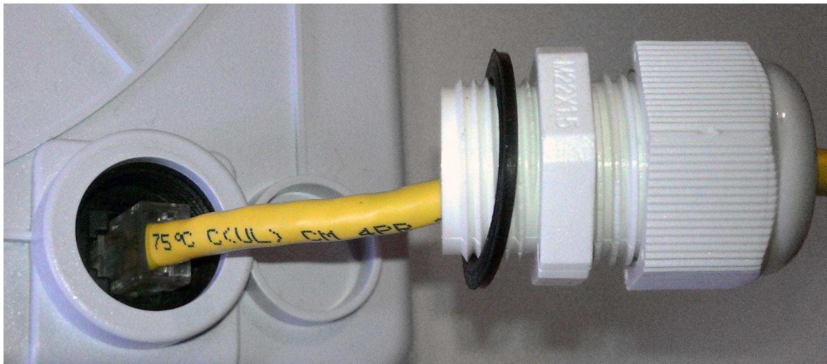
Once the RJ45 connection has been made, screw in the gland into the housing making sure it is tight enough for a water tight seal.
