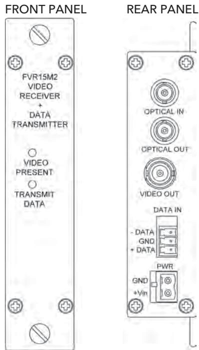
NOTE: Remove Electrical Connector for Rack Mount Units
