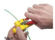
**Blade Replacement:** Replacement blade kit (5 pack): CB 281 p/n 80935 Note: Use caution when handling blades and dispose of used blades properly
